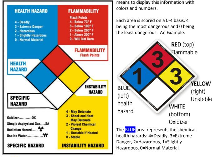
The RED area represents the chemicals fire hazard by using a flash point. 4=A flash point below 73°F, 3=A flash point below 100°F, 2=A flash point above 100°F, 1=A flash point above 200°F, 0=A substance that will not burn
